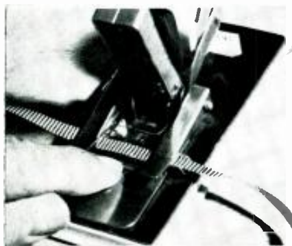
First step in using the kit is to make a loop, splicing the ends together. The lines should match where the splice is made.
