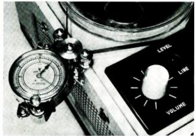
Fig. 6, below, bottom: For strictly limited-use situations, an electric clock fixed up with an easily available on-off switch has genuine possibilities for tape timing. Just turn it on each time you start recording, and off again each time you stop, and you'll have a reasonably accurate indication of how much recording time you've used.
