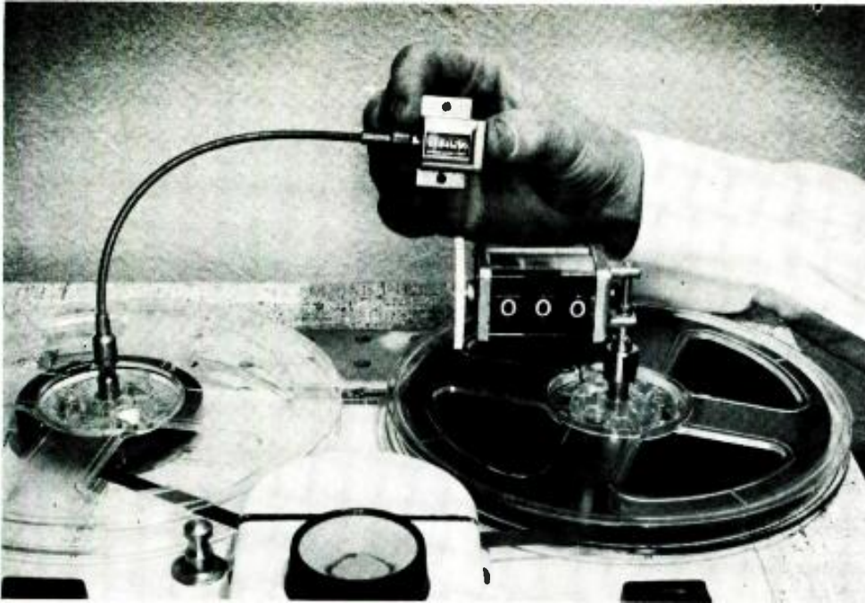
Fig. 4, left: Inexpensive digital revolution counters are available at surplus stores and elsewhere, so perhaps you can put a bit of latent mechanical ingenuity to work figuring out how to add one to your own recorder if it lacks one? This could either be coupled directly to the reel shaft, or coupled via a flexible (removable) cable.
