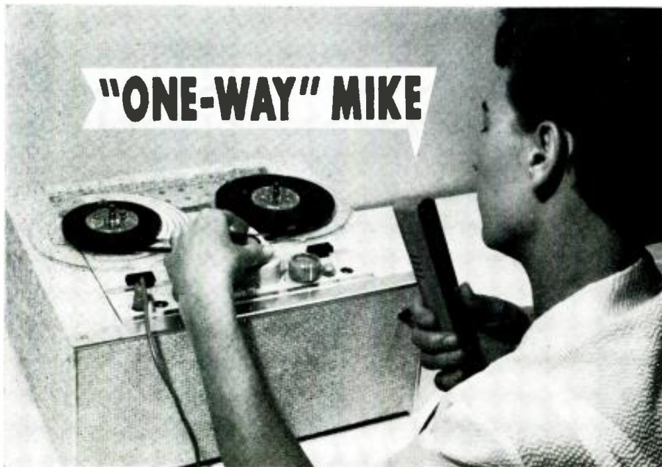
Fig. 11: Because of the split-second accuracy possible when using cueing tabs spotted within an open-faced reel, it's easily possible to add new recordings anywhere IN BETWEEN other recordings, without the usual danger of "running into" (and erasing) them. When working this close to your recorder, a unidirectional (cardioid pattern) microphone will considerably reduce pickup of recorder noise.
